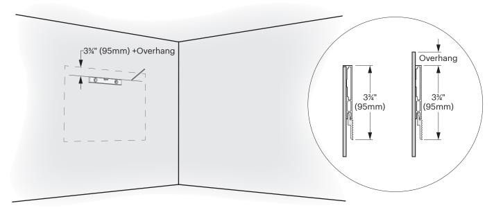
\*If installing multiple Markerboards, determine location of all panels at this time.
