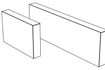
Small 48" W × 31" H × 8" D (1220mm × 785mm × 205mm) Large 96" W × 31" H × 8" D (2440mm × 785mm × 205mm)
