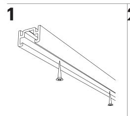
Install the track on the surface using appropriate screws and anchors for the substrate. Space the screws no greater than 16" apart.
