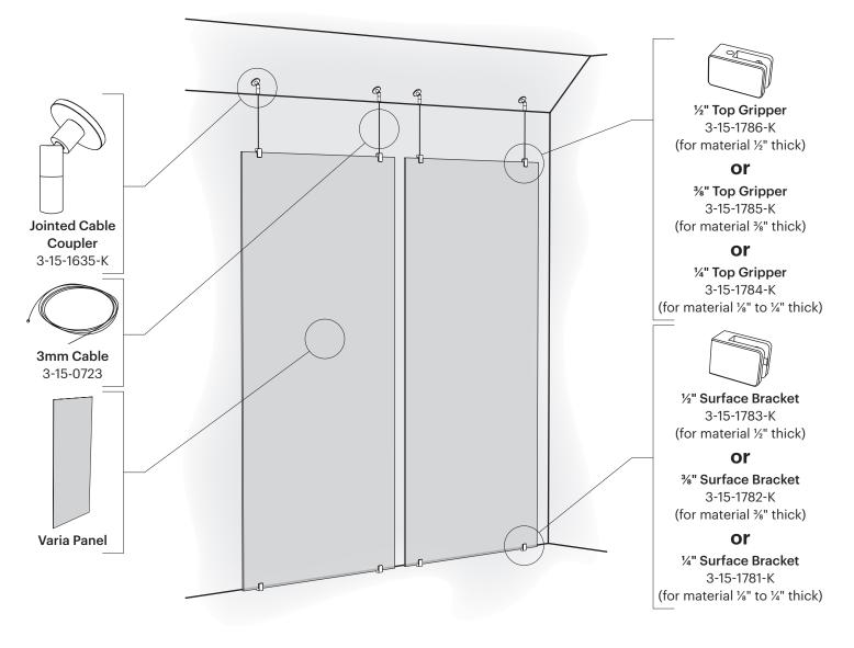
**Note:** With flat panels the weight should always be suspended from the top, not resting on the floor. Otherwise the panels will bow. If the panel is being mounted from the ceiling, as in this solution, the Top Grippers **must** be used with drill thru attachments and not simply set screws.
