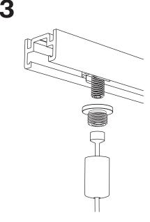
Install the coupler or tensioner without the cover plate.
