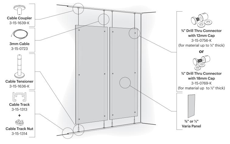
**Note:** The max weight per connector is 25 lbs. Consider this when deciding how many connectors you need for a specific size of panel. Find material weights on the Material Specification Sheets at 3form My Downloads. Also consider panel deflection when determining the number of connections needed for any configuration.
