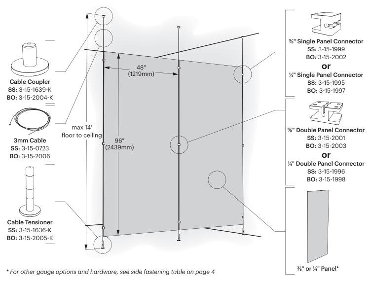
**Note:** You should only anchor Suspend into drywall when you are using a Cable Track on the ceiling or attaching to a wall in a low-traffic area. Any time you fasten cable to drywall you should not exceed 60 lbs. of tension and weight. This means your cable should have some slack, otherwise you risk pulling the anchors out of the drywall. Smooth cable connectors have a maximum weight of 50 lbs per connector.
